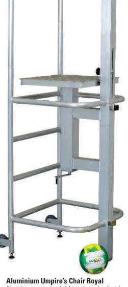
Aluminium construction, height continuously adjustable with crank. Entrance via ladder at rear. Four adjustable rubber feet, webbing for fastening to volleyball post, table and back made of PE500.
