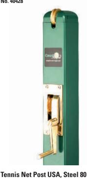
80 x 80 mm galvanized steel, green powder-coated. With brass gear mechanism, stringing block and a removable crank. Ground sleeves not included. Meets the European DIN EN 1510 safety standard.
