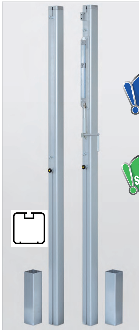
Volleyball Post Universal 80 Aluminium Reliable, solid volleyball post 80 x 80 mm aluminium, compliant with DIN 7896. Easy-running net attachment and tensioning devices (galvanized, trapezoid thread mechanism) continuously adjustable. Surface of the posts and impulse profiles are matt-silver anodized. Complete with ground sleeves and covers. No. 30500
