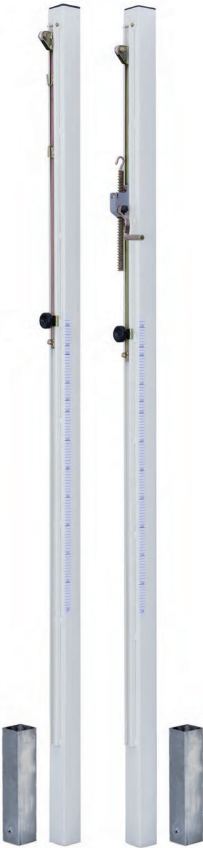
Volleyball Posts Court Royal 80 Steel Very sturdy volleyball posts 80 x 80 mm, made of steel, coated in white. Net attachment and tensioning device galvanized, smooth-running and continuously adjustable. Height of post from the ground 300 cm. Complete with ground sleeves No. 30505
