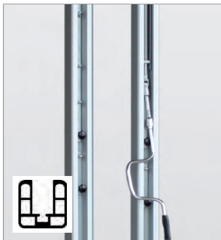
Volleyball post Special 80 Top volleyball post 80 x 80 mm made of aluminium profile compliant with EN 1271. Extra sturdy construction including slider with roller and tensioning device, crank as well as net hooks. Surface matt-silver anodized. Complete with ground sleeves and covers. No. 30520
